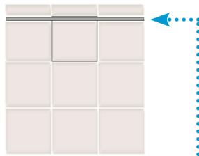
Quick and easy tiling works at line drainage because just one **one slope direction** is required. The channels themselves need a minimum slope to the center.
